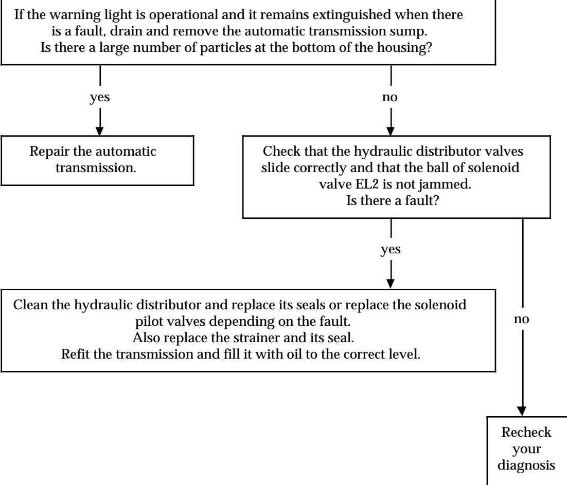
**Chart 2 : Slipping when starting in forward or reverse gear but operating normal above 12.5 mph (20 km/h) in forward gear.**
