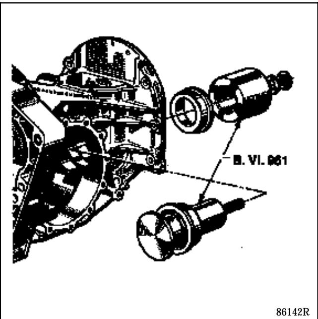
Refit the inner bearing track ring to the final drive pinion (20).
