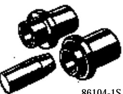
86104-1S     | B. Vi. 951        | 00 00 095 100 | Tool for fitting differential seal                                |
