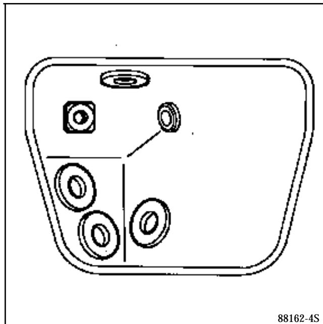
\* Direction for fitting magnets: ribbed side
