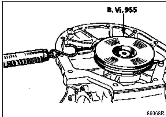
The final drive pinion should rotate under a load of between **2** and **3.5 daN.m.** if the bearings are new and freely, without play, when the original bearings are refitted.
