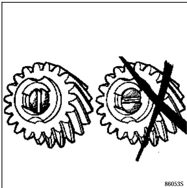
Fitting the differential in the casing.
