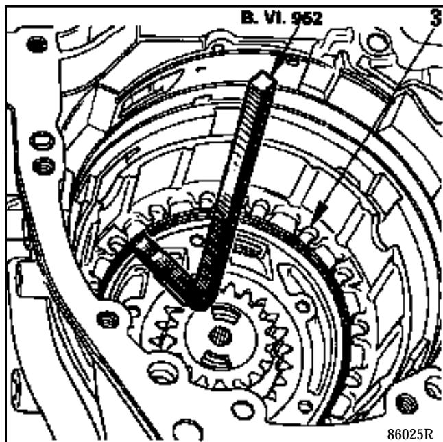
Mark the face (chamfer A) of the oil pump outer pinion and remove (2).
