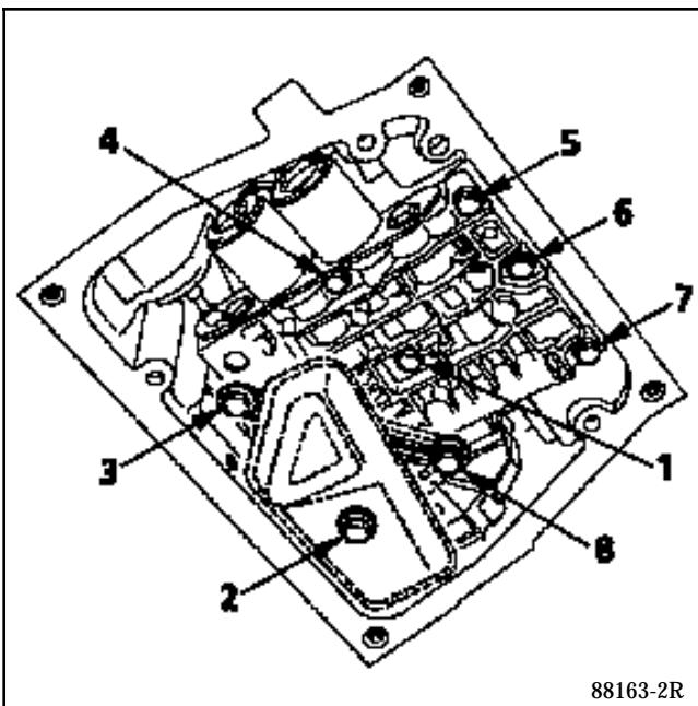
After tightening bolts (1) and (2), fit the new strainer (fitting direction shown in diagram) together with its seal.
