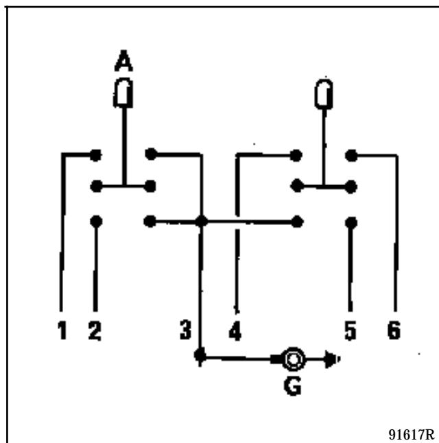
The control pins are represented in the mid position (position D at the lever)
