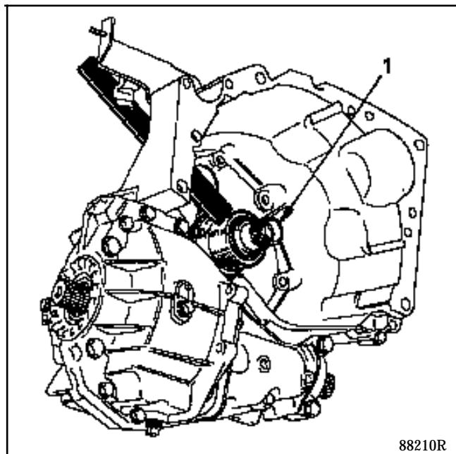
Check the condition of the smooth part of the stator shaft (1).
