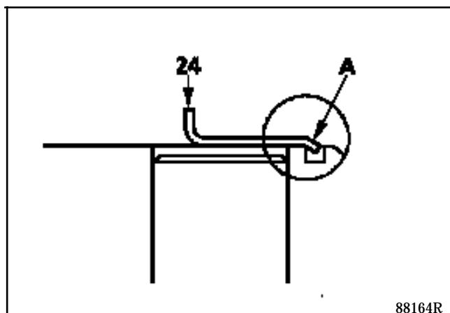
If they are not, move the band ring down slightly using a copper hammer.
