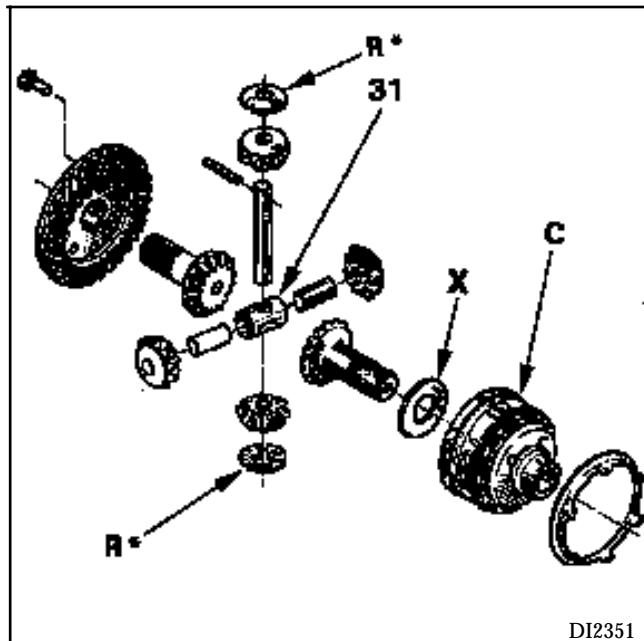
Attach the washers (R) to their respective planet wheels and recover the adjusting shim (X).
