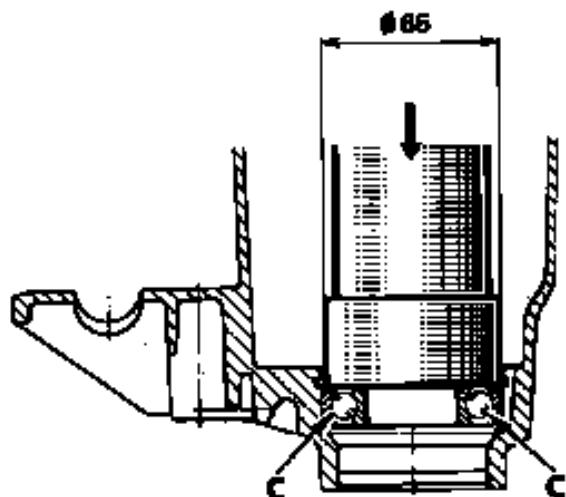
Replace the circlip which holds the bearing.
