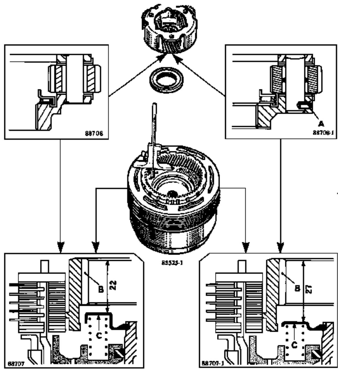
All automatic transmissions of the MB-MJ type before the 85 model may be fitted with the modified E1-E2 assembly - identified by a dimension of **27 mm**. However, it is not possible to fit the strengthened forward gear train to an E1-E2 assembly which has not been modified.
