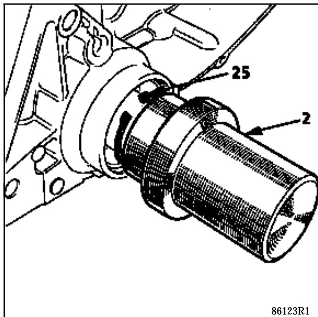
Seal (28) is refitted using tool B. Vi. 945 which consists of:
