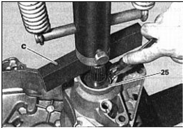
Remove the differential on the press via the sun-wheel with its washer or washers.
