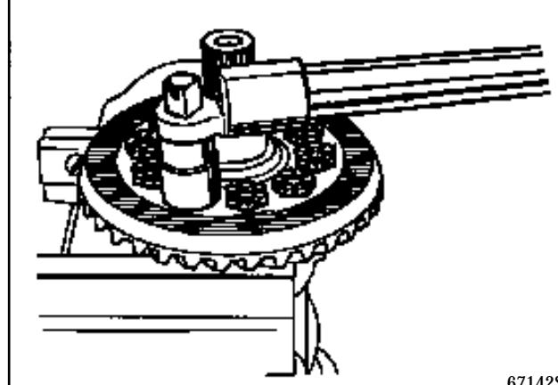
The band ring (24) is refitted on the press using tool **B.Vi. 883**, without the bearing fitted.
