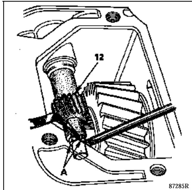
**2nd CASE:** The pinion (12) and the drive wheel (11) are damaged.
