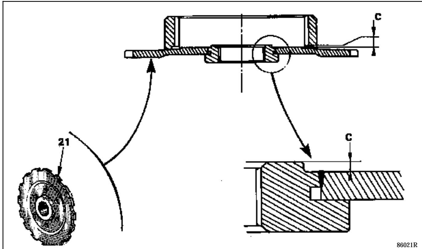
Calculate the thickness E of shim (19).
