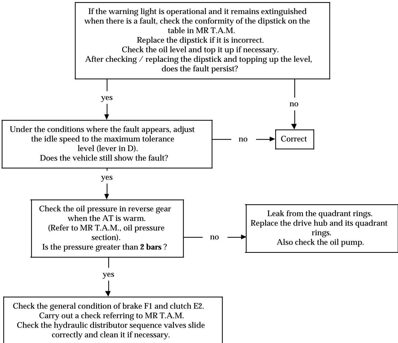
**Chart 6 : The engine races in full load position when changing from 2/3 and 3/1. The automatic transmission seems to change into neutral.**
