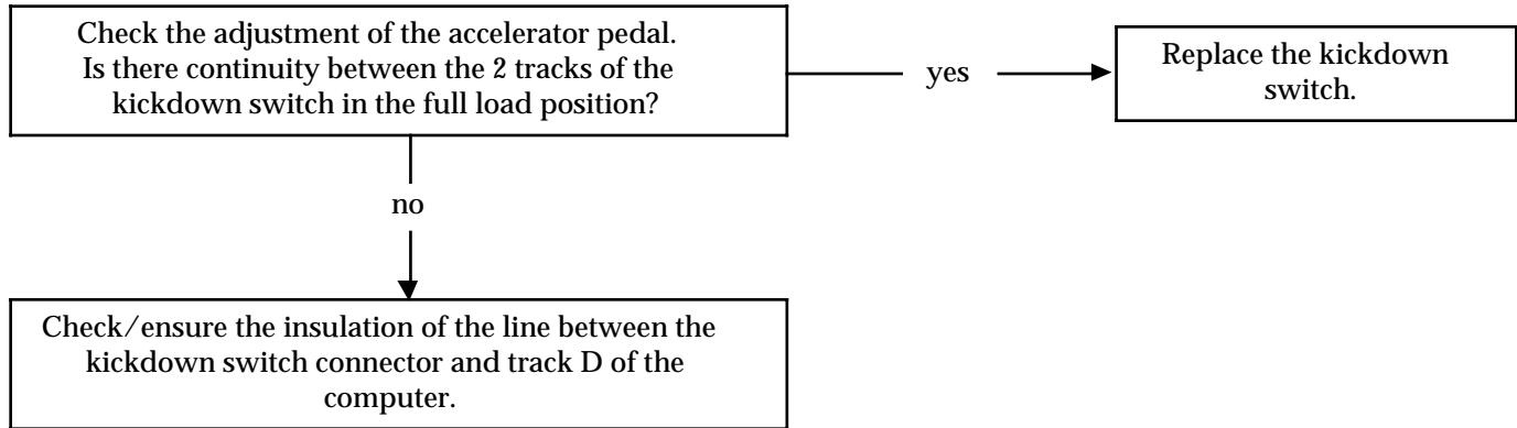
Vehicles fitted with a closed contact kickdown switch:
