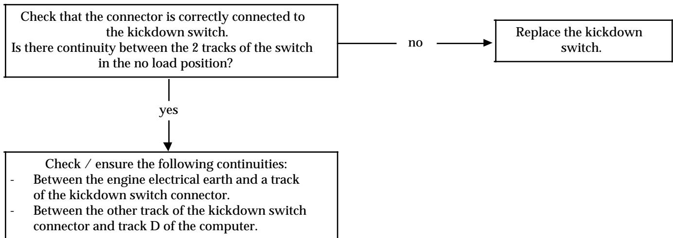
Vehicles fitted with a closed contact kickdown switch:
