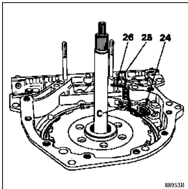
**NOTE:** to limit the movement of the park pawl (24), there is a shim which is placed between the park pawl and the gear section at (C).
