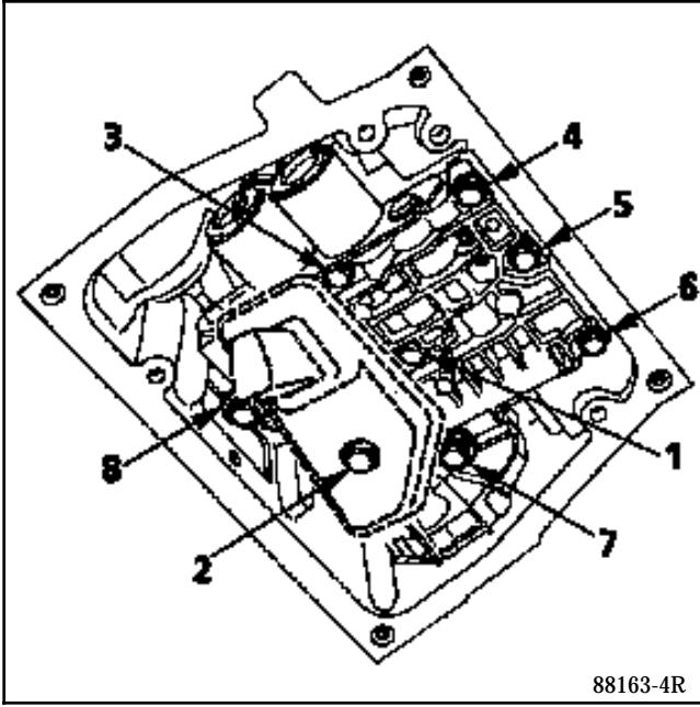
After tightening bolts (1) to (6), fit the new strainer (fitting direction shown in diagram) together with its seal.
